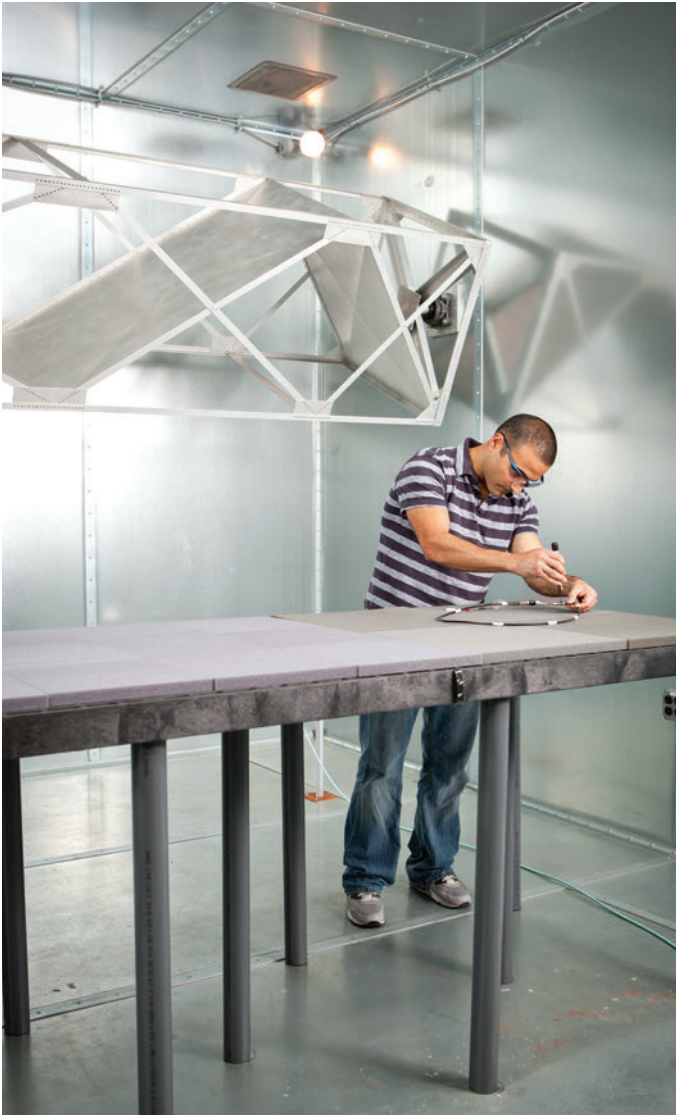
Mode stir RF-Shielding testing per IEC Standard 61000-4-21 Annex F
